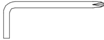
L type hexagon socket wrench (5×30×85) 1 pc
