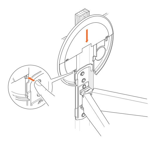
4. Slide the **wall plate cover** (S) onto the **wall mount** (A). To remove the cover plate, press the left tab and slide it off the wall mount.
