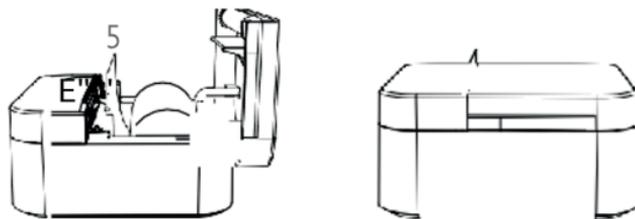
Open the cover in the direction of the arrow as shown in the figure, and pull up the paper compartment cover to open the cover. Put the paper in the printer the direction shown in the figure, put the heat-sensitive surface of the paper on the same side as the heat-sensitive head.
