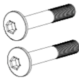
Allen socket full thread screw M8×50×20 * 2 PCS
