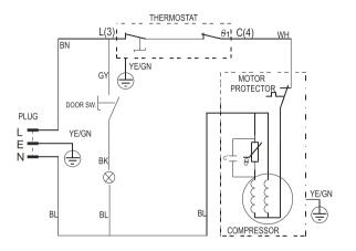
C\*: The capacitor is optional according to different compressor model.
