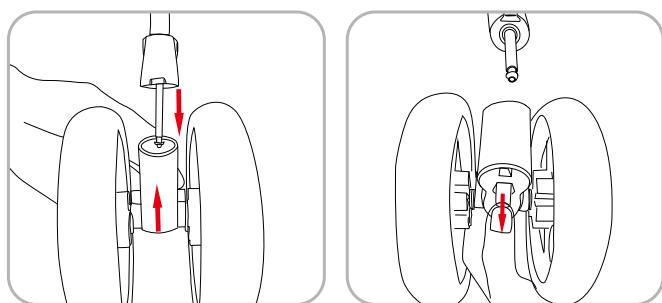
1. Install and disassemble front wheels: Insert the front wheel set into the front wheel seat, it is installed when hear "Click". Press the buckle on the front wheel seat with your hand and pull it down, then the front wheel set is removed.
