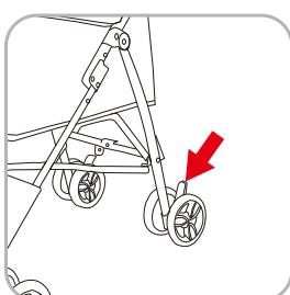
A. Braking: Press down the rear wheel brake levers on both sides
