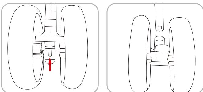
2. Install & disassemble rear wheels : Insert the rear wheel set into the rear wheel seat, it is installed when the barb on the rear wheel seat pops out .Hold the barb on the rear wheel seat and pull it out, the rear wheel set can be removed.
