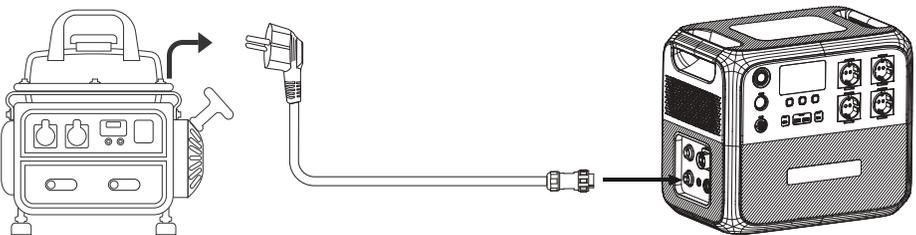
**Note:** Make sure your generator delivers the AC output with charging voltage, frequency, and Grid Self-adaption Mode voltage that meet AC200P L's specifications.
