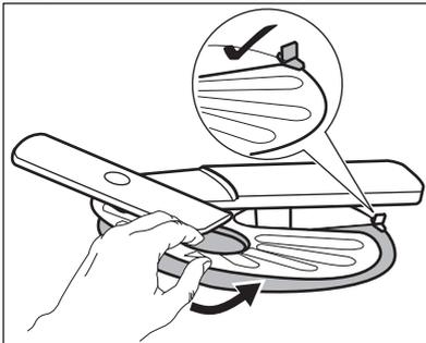
7. Reassemble the filters (B) and (C).
