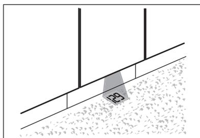
TimeBeam displays the following information on the floor below the appliance door:
