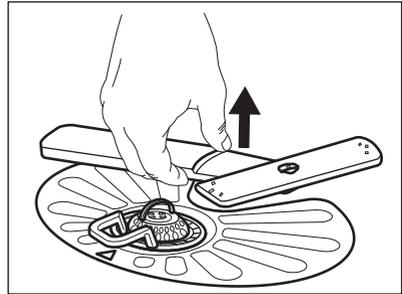
2. Wash the spray arm under running water. Use a thin pointed tool, e.g. a toothpick, to remove particles of soil from the holes.
