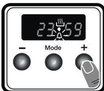
2. Select the desired time period using the "+" and "-" keys while
