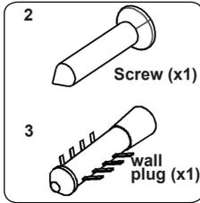
The document bag contains an anti-tilting kit. Loosely attach the anti-tilting bracket (1) to the wall using the screw (2) and wall plug (3), following the measurements shown in the figure and table below. Adjust the height of the anti-tilting bracket so that it lines up with the slot on the cooker and tighten the screw. Push the appliance towards the wall making sure that the anti-tilting bracket is inserted into the slot on the rear of the appliance.
