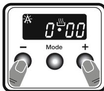
1. Press the "+" and "-" keys simultaneously.
