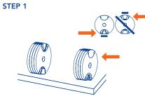
Unpack and prepare two symmetrical **Stacks (A)** of connected weight plates on a flat surface, making sure that each stack has an **End plate (B)** with a **Flat connector (C)** pointing outwards. The flat side of the stack should point downwards.
