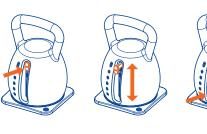
Place the KETTLEBELL in the base unit. Female and Male connector must be aligned. Try pushing the switch knob to unlock (extend), choose the preferred by shifting adjuster up or down. Then push in again to lock the weight you want.
