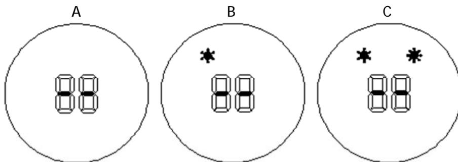
3. Turn-off timer. Press button to set timer (1-12hours) during working status. Pressing the button one time increases one hour for timer. After setting time, the display will show current setting time for 5 seconds, then resume to previous display, meanwhile the light on. Below photo is an example of setting 8h.
