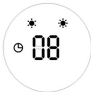
4. Turn-on timer. In standby mode, press timer button, you can set the appointment turn-on time in 1-12 hours. After complete setting, the display shows the appointment turn-on time and also the light is on. The display automatically decreases 1 hour for each hour passed. When the appointment power-on time arrived, the product will automatically turns on. The default setting temperature is 23 °C during appointment turn-on. Below photos is an example to set appointment turn-on time to 8 hours:
