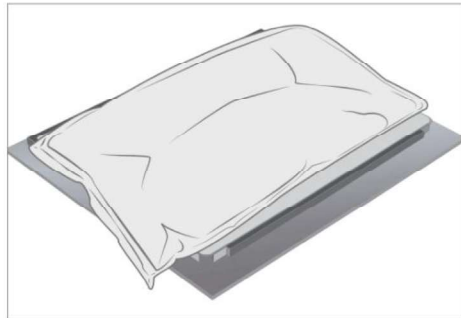
Place 9 kg steel shot bag onto device
