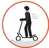
EN Keep your speed between 3.1-6.2mph (5-10 km/h) when you ride through speed bumps or other uneven surfaces.
