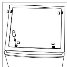
2. Unscrew and remove the hinge. Then lift lower door and place it on a soft pad to avoid scratch.
