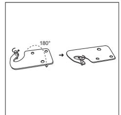
11. Place the upper door back on. Ensure the door is aligned horizontally and vertically so that the seal are closed on all sides before finally tightening the top hinge. Then inert the hinge and screw into the front of the unit.
