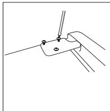
3. Unscrew middle hinge. Then lift lower door and place it on a soft pad to avoid scratch.
