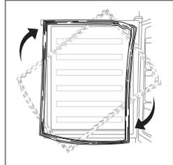
9. Make the middle hinge reverse the direction 180°, the transfer it to the left property position. Place the lower door back on. Make the middle hinge pin in the upper hole of the lower door, then tight the bolts.
