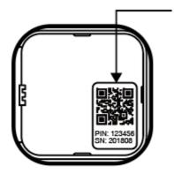
**Note:** QR Code used for SmartStart inclusion. DSK Code can be found on packaging. Do not remove or damage them.
