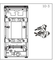
2. Fill the 4 left holes with blanking plugs (Fig. 10-4).
