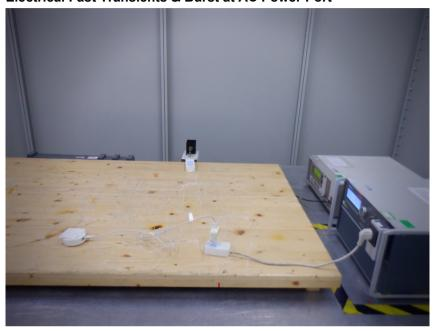
**Electrical Fast Transients & Burst at Signal Port**
