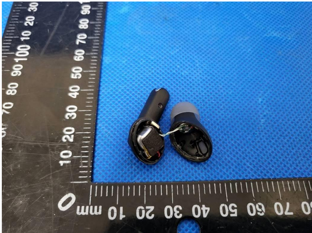
Fig. 18 Internal view of earbuds_left side
