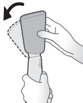
Note: At the default position, the steamer head is at uplift position. Do not adjust the steamer head when steamer head is hot.
