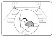
**1.** Open the door and flip open the clips at both hinges.
