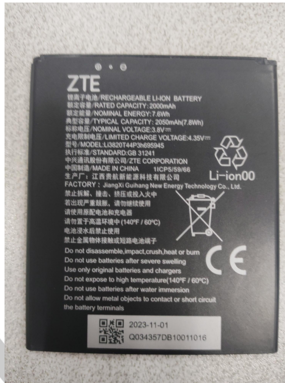
Battery (Li3820T44P3h695945 3.8V 2000mAh 7.6Wh)
